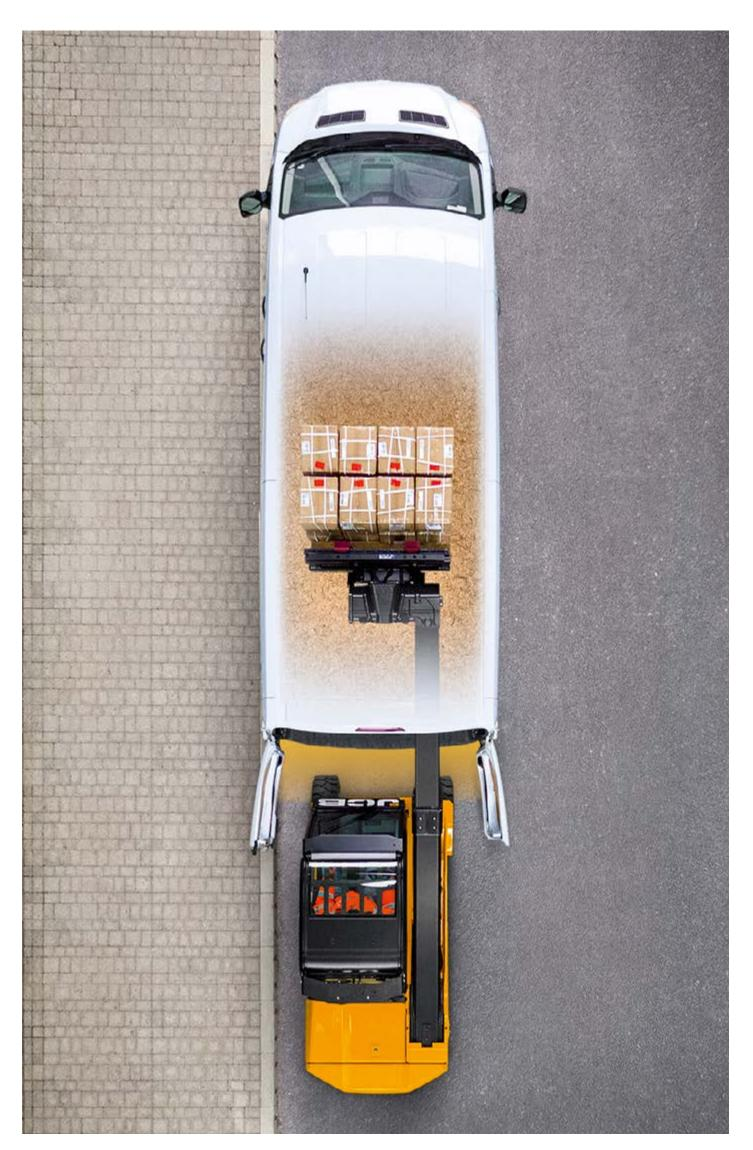
Save 70m<sup>2</sup> of space per truck with single side loading. Unique forward reach allows you to load and unload trucks from one side in indoor and outdoor environments, saving valuable space, time and money.
